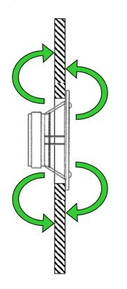
Stop of acoustic short-circuit with closed cabinet
