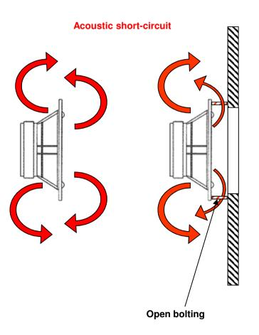
Stop of acoustic short-circuit with baffle
